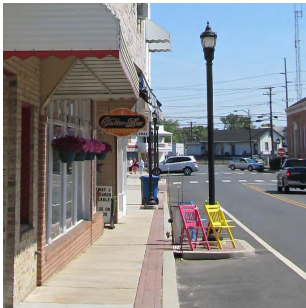
Curb bump-outs and on-street parking are effective traffic calming measures. A Downtown business has chosen to decorate this particular bump-out with a colorful display of furniture, further adding to the appeal of the adjacent store, while still maintaining a free-flowing pedestrian walkway.
